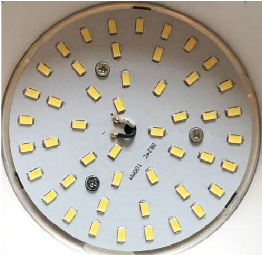
Picture 5. model: B0104-24-Y-1-Z, B0104-24-Y-3-Z LED module view
