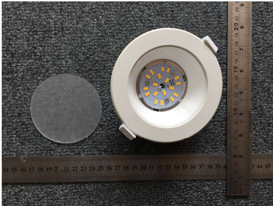
Picture 17. model: B0104-12-Y-1-Z, B0104-12-Y-3-Z internal view (I)
