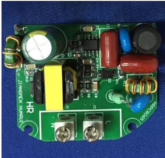
Picture 13. model: B0104-15-Y-1-Z LED driver view
