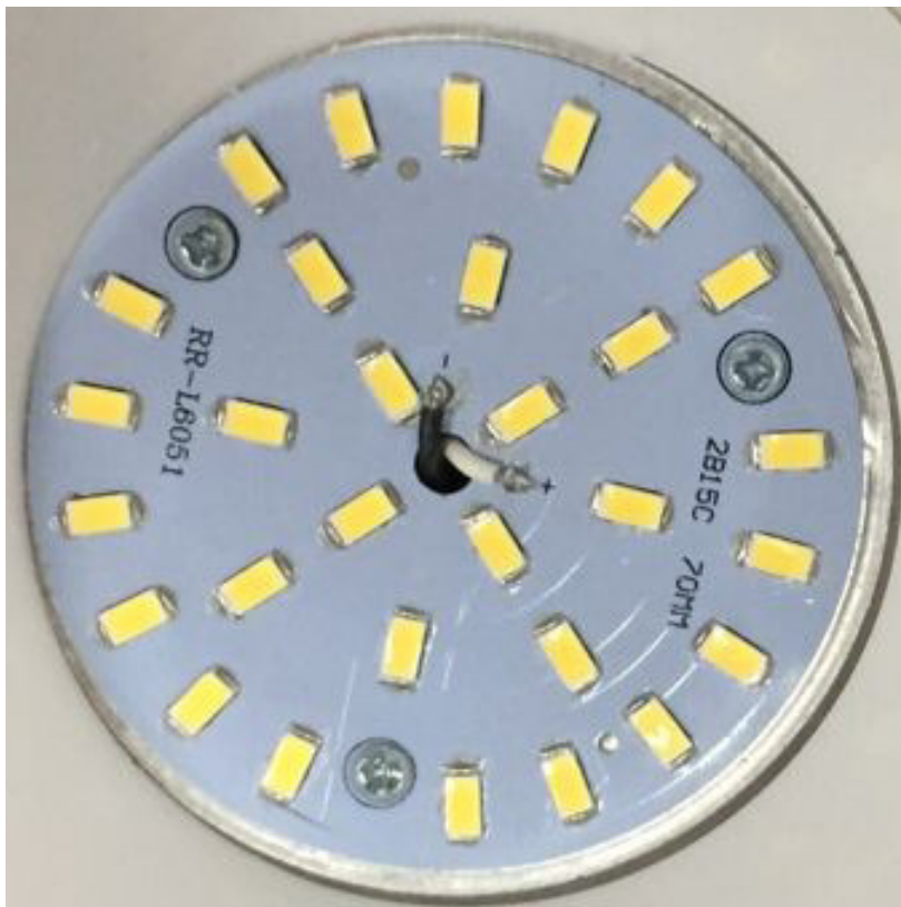
Picture 12. model: B0104-15-Y-1-Z, B0104-15-Y-3-Z LED module view
